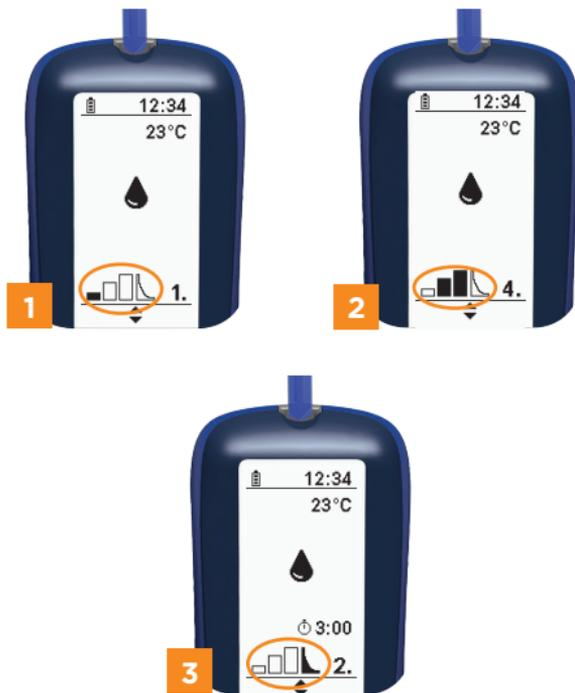
You can begin with any of the step test phases. However, you cannot change the order of the test step phases. As an example, pre-exertion cannot be selected after the exertion phase.
